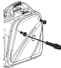
Figure 4-3. Remove Side Cover
