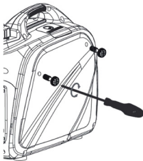
Figure 2-8. Remove Side Cover
