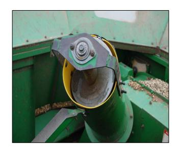
Now install the 10-24 x 3/4" Phillips head screw supplied at the location shown below.
