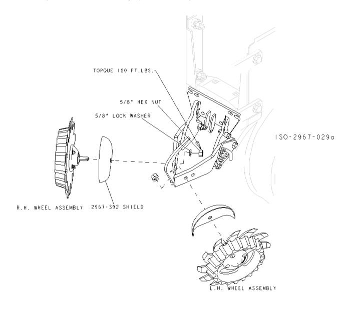
Regularly inspect the residue manager for loose or worn parts. Repair and replace as needed.
