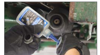
Apply thread locker.
