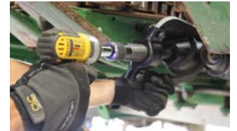
Extend hydraulic puller.
