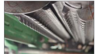
Ensure cutting flutes remain intermeshed.
