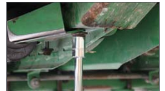
Replace bolts in trash knives.
