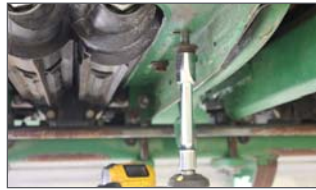
Remove bolts from trash knives.
