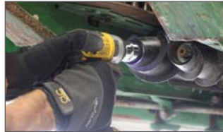
Remove front-end nut from drive shafts.
