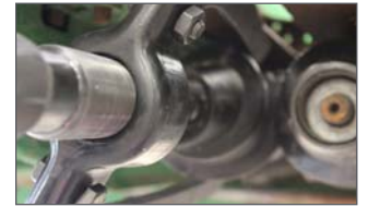
Attach puller arms to pulling features on castings.
