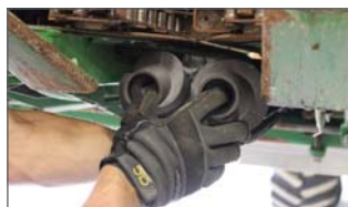
Lift rolls together and place rolls on drive shafts.
