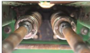
Put male keys in an X pattern.
