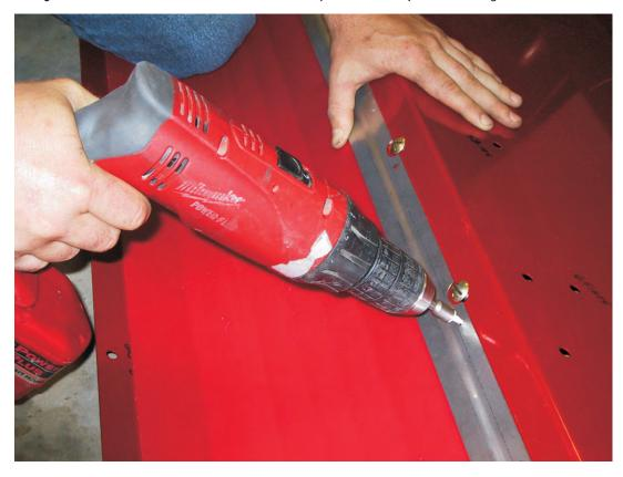
Step 6 With the "Upper Rear" hold-down in place, install the "Upper Front Left" and "Upper Front Right" hold-down strips in a similar manner. NOTE: Take care to position the front strips parallel to the rear strip.
