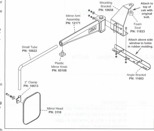
6. Insert the small tube into the mirror arm assembly and secure with the plastic mirror knob.
