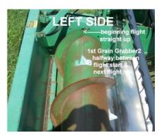
1. To begin, roll auger in direction of travel until outer end flight beginning point is at 12 o'clock noon.
