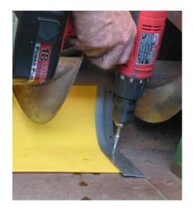
IMPORTANT: WITH THE END CAP FASTENED IN PLACE AND THE AUGER BEARING SUPPORT PLATE RE-ASSEMBLED AND CENTERED, MANUALLY ROTATE THE AUGER TO CHECK CLEARANCE BETWEEN THE END CAP AND THE AUGER FLIGHT. IF THE AUGER MAKES CONTACT WITH THE END CAP OR FASTENERS, AND YOU CAN NOT RAISE THE AUGER BY LOOSENING AND RAISING THE BEARING SUPPORT PLATE, STOP INSTALLATION AND CALL CUSTOMER SERVICE @ 1-800-542-7659.
