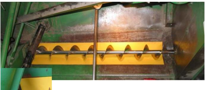
5. SLIDE THE LINER TO THE LEFT UNTIL IT MAKES CONTACT WITH THE SUPPORT FLANGE OF THE VERTICAL AUGER HOUSING, THEN CENTER THE LINER WITH THE AUGER AS ILLUSTRATED ABOVE.
