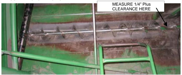
4. STARTING WITH THE FRONT (LOWER) AUGER, INSERT THE SHORTER POLY LINER UNDER THE AUGER.
