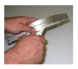
9. WHILE HOLDING PRESSURE IN THE BOTTOM / CENTER, SECURE THE END CAP IN PLACE STARTING WITH THE CENTER HOLES AND WORKING OUTWARD.
