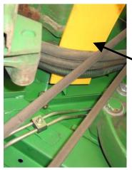
IMPORTANT: PRIOR TO DRILLING AND/OR SECURING THE END CAP IN STEPS 8 AND 9, INSERT THE 4" X 6" PLASTIC "DRILL SHIELD" SUPPLIED AS ILLUSTRATED TO PREVENT DRILLING INTO THE ELECTRICAL HARNESS OR RUBBER HOSES LOCATED ON THE UNDERSIDE.
