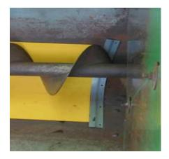
7. TEST FIT THE END CAP ON THE RIGHT END OF THE LINER. THE END CAP SHOULD FIT BELOW AND ADJACENT TO THE SUPPORT FLANGE OF THE CLEAN ELEVATOR HOUSING.
