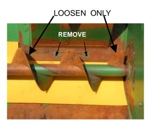
13. REMOVE THE (2) INNER BOLTS AND LOOSEN ONLY THE (2) OUTER BOLTS ON THE ELEVATOR HOUSING FLANGE AS ILLUSTRATED.
