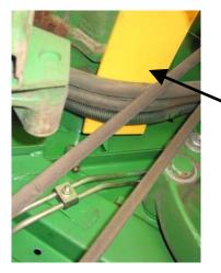
NOT THE END CAP IN STEPS 8 AND 9, INSERT THE 4" X 6" PLASTIC "DRILL SHIELD" SUPPLIED AS ILLUSTRATED TO PREVENT DRILLING INTO THE ELECTRICAL HARNESS OR RUBBER HOSES LOCATED ON THE UNDERSIDE.
