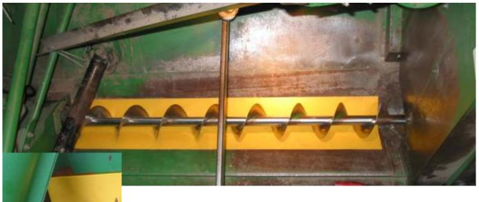
5. SLIDE THE LINER TO THE LEFT UNTIL IT MAKES CONTACT WITH THE SUPPORT FLANGE OF THE VERTICAL AUGER
