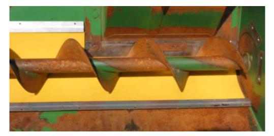
16. COMPLETE THE INSTALLATION BY SEALING THE RIGHT END OF THE LINER WITH SILICONE SEALANT.
