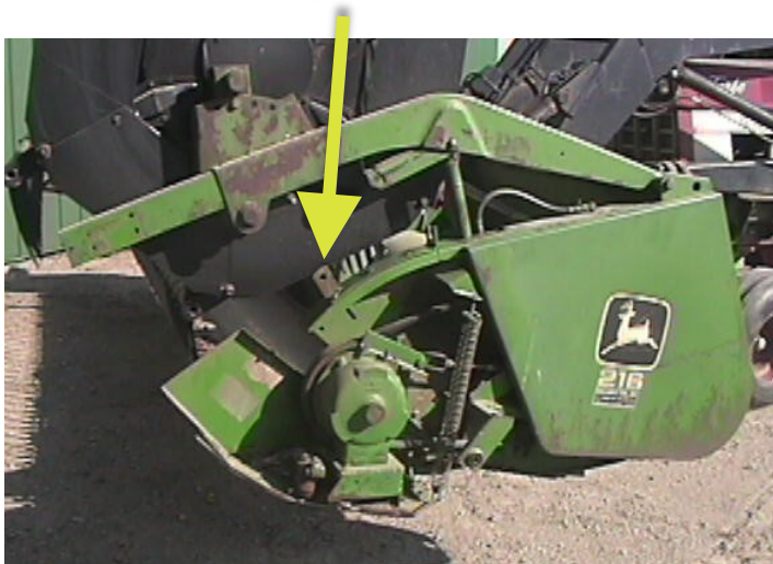
View after removal of old divider, spring and brackets.
