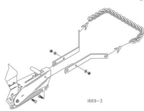
**STYLE 3.** Attaching drag chain kit to closing wheel arm with holes provided. Attach brackets as shown in drawing to the left using 3/8" x 1" hex bolt, flat washer and locknut. Securely tighten hardware.
