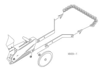
**STYLE 2.** Attaching drag chain kit to closing wheel arm without holes or bolt on wheels. Drill a 13/32" hole on each side of arm. Locate hole as shown in drawing to the right. Using 3/8" x 1" hex bolt, flat washer and locknut, attach brackets as shown.
