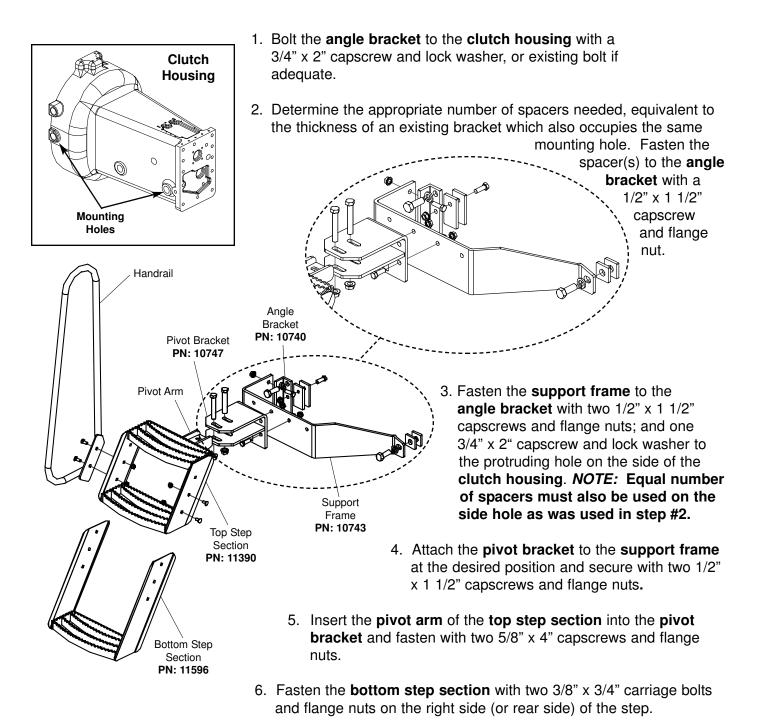
7. Use two 3/8" x 1" carriage bolts and flange nuts on the left side (or front side); also include the **handrail** at this location.
