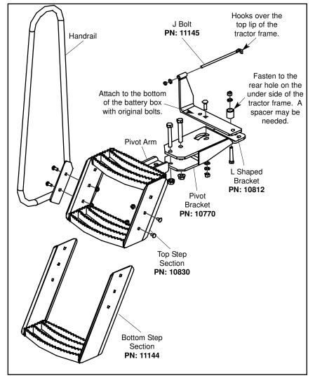
The bolt length used will depend on the spacer that is required.
