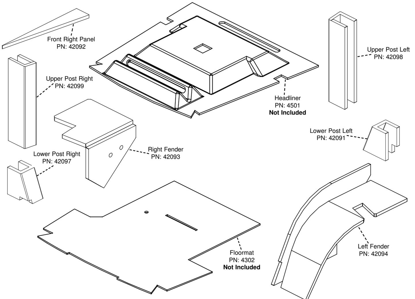
1. To make installation of your new cab foam kit easier, remove seat to allow more room to work. Also remove floor mat, ashtray, radio, AC and heater controls and vents in models where necessary.
