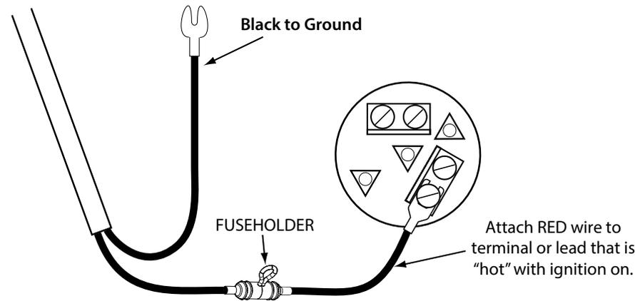
2-amp in-line fuse required (Not Provided) for unprotected circuits
