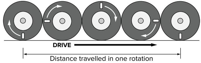
To determine SPEED CAL, measure the distance of one complete wheel revolution and divide by the number of magnets installed.
