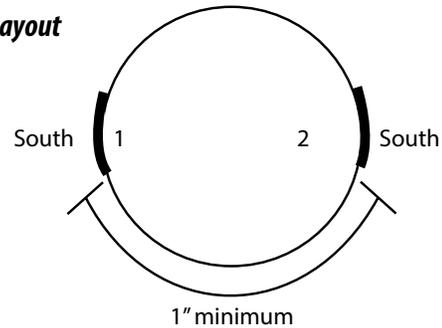
**NOTE: Magnets can be placed closer than 1" apart if a magnet with opposite polarity is placed between them.**
