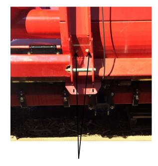
From behind the head drill 3/8 holes thru the liner where you removed bolts that connect the floor panel to the frame at either side of the throat. Install 5/16x 1" carriage Bolts as shown in picture to the right.
