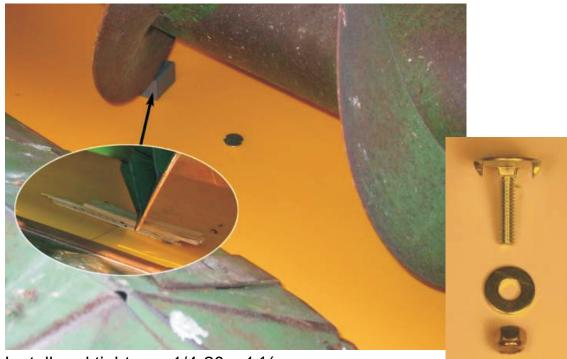
12. Install and tighten a 1/4-20 x 1 <sup>1</sup>/<sub>4</sub> fanged bolt in the center hole.
