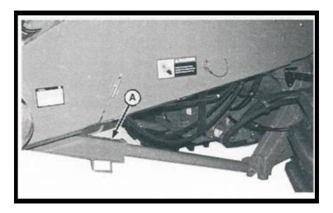
10. With the corn head raised and secured, measure the underside of the head from left to right and mark the mid-point as illustrated below:
