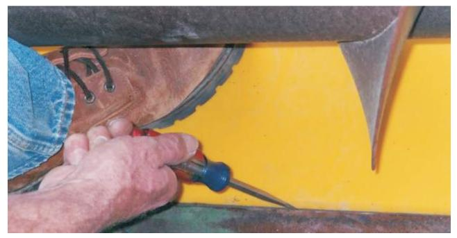
NOTE: IT IS VERY IMPORTANT THAT THE LEADING EDGE OF THE POLY PANEL "SNAPS" INTO PLACE BEHIND AND UNDER THE STEEL PLATE AT EACH ROW.
