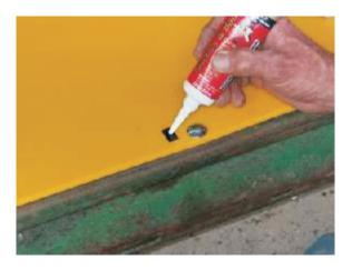
Use the silicone sealant supplied to seal around each bolt head and to fill in any unused holes. 9. With the wooden shims still in place, attach the header to the combine.
