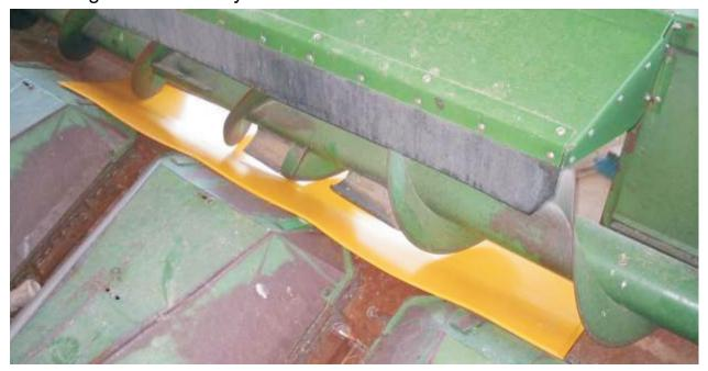
5. With the Poly panel pushed fully to the rear and the rear mounting holes aligned, pry the front edge of the panel behind and under the steel plate at each row with a large screw driver or pry bar.
