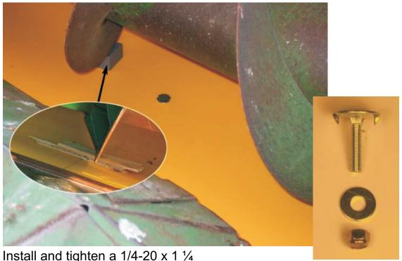
12. Install and tighten a 1/4-20 x 1 ¼ fanged bolt in the center hole.
