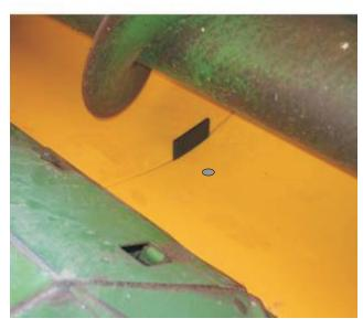
17. To complete the installation, (working from the center outward), layout and drill each panel from underneath the header using the Recommended Hole Location guide below.
