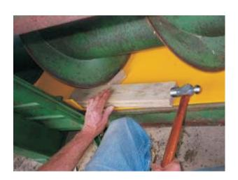
15. Using the black 3/16" gauge, position the panels so there is a 3/16" gap at each joint as illustrated below.
