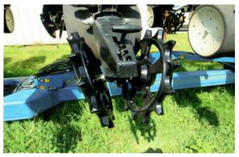
For optimal performance, Furrow Cruisers should run in pairs.
