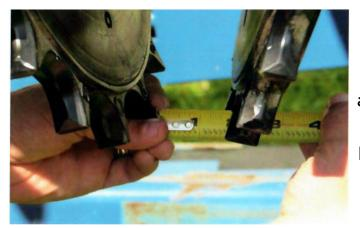
In high contour planting and turning on side hulls, install the Furrow Cruisers in the front holes and widen them to approximately 1 1/2 inches apart. This will help in keeping the spike out of the furrow and on the sidewall
