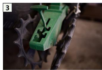
Install Furrow Cruisers in the back holes of the tailpiece straight across from each other.
